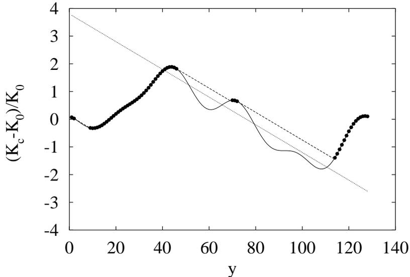
Fig. 4. Schematic construction for the strong pinning case. The continuous curve shows the local toughness profile. In contrast to the previous figure, many solutions of equilibrium position exist as shown by the five intersections of the dotted line with the continuous curve (three stable positions and two unstable ones). This selects only a subset of accessible arrest sites shown by bold dots, separated by sudden jumps shown by a dashed line of slope  $-S$ .
