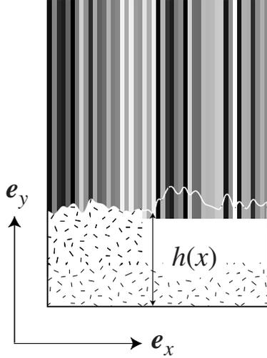
Fig. 1. Crack propagation in a layered toughness configuration. The crack front is distorted such that at every point  $x$  along the front the stress intensity factor  $K(x)$  matches exactly the local toughness value  $K_c(x)$ .
