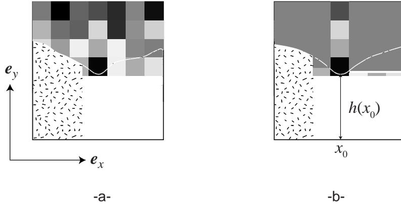
Fig. 2. A random toughness configuration is represented schematically on the left (a) with a grey-scale coded toughness. On the right, (b), a reference case is constructed by extracting the toughness pattern along a line parallel to the propagation direction, and substituting to the rest a uniform toughness environment. The latter is determined such that the deflection  $\Delta h = h(x_0) - \langle h(x) \rangle_x$  is zero on average over all accessible crack front conformations.
