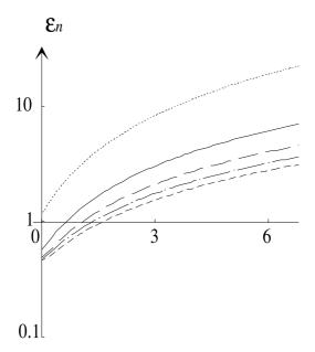
Figure 3: Logarithmic plot of  $\varepsilon_1$ , ...,  $\varepsilon_5$ , against the parameter  $\alpha$  that determines the strength of the exterior field. The rescaled magnetic induction is m=1, and the angle between the propagation direction and the exterior field is  $\theta=\pi/4$ . The legend is the same as in figure 1.
