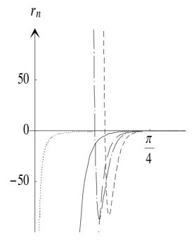
Figure 1: Plot of the five first time scaling coefficients  $r_1$ , ...,  $r_5$  against the angle  $\theta$  between the propagation direction and the exterior field. The rescaled magnetic induction is m=1, and the parameter determining the strength of the exterior field is  $\alpha=0.5$ . Dotted line:  $r_1$ , solid line:  $r_2$ , large dashing:  $r_3$ , dashed-dotted line:  $r_4$ , short dashing:  $r_5$ .
