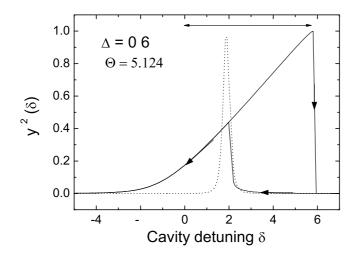
Fig. 8. Same calculation as in Fig. 7 performed here for stronger thermal effects corresponding to  $P_{cm}=5.7\,\mathrm{W}$ , with  $P_{\omega}^{\mathrm{abs}}=17\,\mathrm{mW}$  and  $P_{2\omega}^{\mathrm{abs}}=128\,\mathrm{mW}$  ( $L_c=10\,\mathrm{mm}$ ,  $w_0=20\,\mu\mathrm{m}$ ). The dotted line would be the sharp fringe observed on the reverse scan direction.
