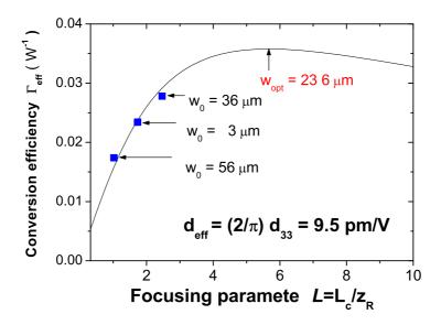
Fig. 3. Conversion efficiencies  $\Gamma_{\rm eff}$  versus the focusing parameter  $L=L_c/z_R$ . The 3 squares are the experimental points measured at  $w_0=56,43,36\,\mu{\rm m}$  and the solid line are the theoretical values from Eqs.(5)-(6) using the labelled value of  $d_{\rm eff}$  after optimisation of the focusing function h over the mismatch parameter  $\sigma$ . The theoretical optimal waist is found at  $w_{\rm opt}=23.6\,\mu{\rm m}$ .
