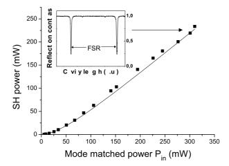
Fig. 5. SH power versus the mode-matched FF power. The solid line is a calculation from Eq. (3) making use of  $\epsilon = 0.021$ ,  $T_1 = 0.12$ ,  $\Gamma = 0.023 \,\mathrm{W}^{-1}$ . The inset shows the FF reflection fringe contrast at maximum power.
