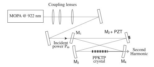
Fig. 2. Schematic of the experimental setup.
