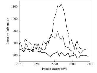
FIG. 1: Mo L $\alpha$  emission for various electron energies close to and below the Mo  $2p_{3/2}$  threshold (2520 eV). Solid line : 2515 eV; dotted line : 2525 eV; dashed line : 2535 eV.
