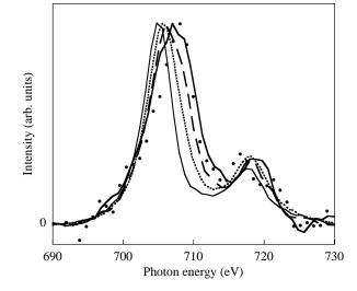
FIG. 13: Fe L $\alpha$  and L $\beta$  emissions of Fe metal, obtained with 2508 eV (thin solid line), 1208 eV (dotted line), 828 eV (dashedline), 758 eV (thick solid line), and 743 eV (dots) electrons.
