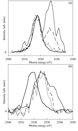
FIG. 3: Mo L $\beta_2$  emission of Mo metal for various electron energies. (a) Thick solid line : 6015 eV; dotted line : 3015 eV; dashed line : 2665 eV; thin solid line : 2630 eV. (b) Thick solid line : 3015 eV; dotted line : 2565 eV; dashed line : 2555 eV; thin solid line : 2535 eV.
