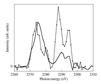
FIG. 14: W  $\rm M_3O_5$  emission of W metal, obtained with 2805 eV (dashed-dotted line), and 5515 eV (solid line) electrons.
