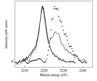
FIG. 9: Zr L $\beta_2$  emission of Zr metal, obtained with 2285 eV (dots), 2515 eV (dotted line), and 5015 eV (solid line) electrons.
