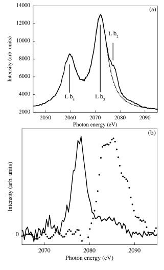
FIG. 8: Y L $\beta_2$  photon energy range of Y metal. (a) Original spectrum obtained with 4815 eV electrons (solid line), and fit of the L $\beta_{3,4}$  doublet (dotted line). (b) Treated spectrum obtained with 4815 eV electrons (line), and spectrum obtained with 2365 eV electrons (dots).
