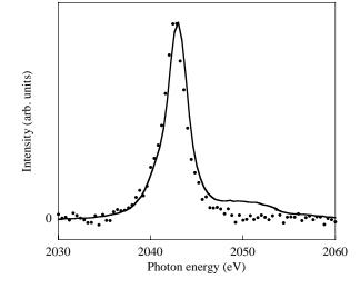
FIG. 10:  $\operatorname{Zr} L\alpha$  emission of  $\operatorname{Zr}$  metal, obtained with 2285 eV (dots), and 5015 eV (line) electrons.
