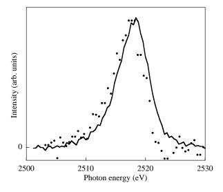
FIG. 6: Mo L $\beta_2$  emission of Mo<sub>5</sub>Si<sub>3</sub>, obtained with 2815 (dots), and 6015 eV (line) electrons.
