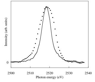
FIG. 4: Mo  $L\beta_2$  emission obtained with 6015 eV electrons on Mo metal (line), and the oxide MoO<sub>3</sub> (dots).
