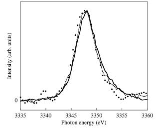
FIG. 12: Ag L $\beta_2$  emission of Ag metal, obtained with 3505 eV (dots), 3795 eV (dotted line), and 7515 eV (solid line) electrons.
