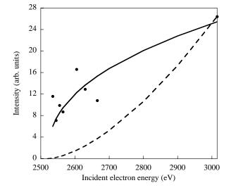
FIG. 5: Power law fit (solid line) of the intensity of the satellite line of the Mo  $L\beta_2$  emission as a function of the electron energy (dots). The dashed line is a power law with the same exponent (1.6) as that of the normal line.
