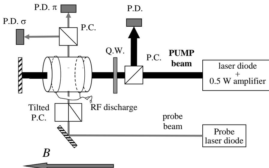
Fig. 3. The main elements of the OP experiment are shown (not to scale). The pump beam, parallel to the magnetic field  $B$ , is circularly polarised using a linear polarising cube (P.C.) and a quarter-wave plate (Q.W.). The absorption of the pump beam is monitored by a photodiode (P.D.) after a double pass through the cell. The transverse probe beam is prepared with  $\sigma$  and  $\pi$  polarisation components which are separated after crossing the cell and simultaneously recorded.
