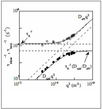
Figure 7 C12-sample:  $q^2$  -dependence of the inverse of the fast (open circles) and slow (full circles) relaxation time. The solid lines are the simultaneous fit to the data of Eqs. (3). The fitting parameters are given in table 2. The dashed lines are the asymptotic behavior at small or large values of  $q^2$ .
