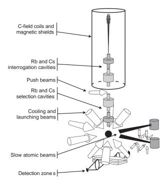
FIG. 1: Schematic of the double fountain both base on  $^{87}$ Rb and  $^{133}$ Cs, so that there is two pairs of cavity finely tuned on hyperfine atomic frequency of corresponding atoms and two ovens. On the cesium part, a transversal collimation of the atomic beam has been improved in addition of the present chirp cooling. This consists in a 2D recycling light, pair of laser beam, used in a "zigzag" way. This allows to load around  $10^9$  atoms in 200 ms in an optical molasses.
