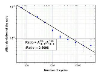
FIG. 3: Allan deviation of the ratio of atom numbers in the  $|4;0\rangle$  obtained by alternating each 60 fountain cycle a full atom number configuration over half atom number configuration on the  $|4;0\rangle$  state as a function of cycle number. The Allan deviation of the ratio averages as white noise and reaches  $\sim 10^{-3}$  resolution after 1 hour. It leads to evaluate AP at the  $10^{-3}$  level.
