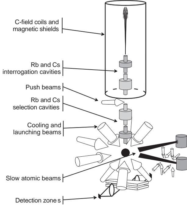
FIG. 1: Schematic of the double fountain both base on  $^{87}\text{Rb}$  and  $^{133}\text{Cs}$ , so that there is two pairs of cavity finely tuned on hyperfine atomic frequency of corresponding atoms and two ovens. On the cesium part, a transversal collimation of the atomic beam has been improved in addition of the present chirp cooling. This consists in a 2D recycling light, pair of laser beam, used in a “zigzag” way. This allows to load around  $10^9$  atoms in 200 ms in an optical molasses.
