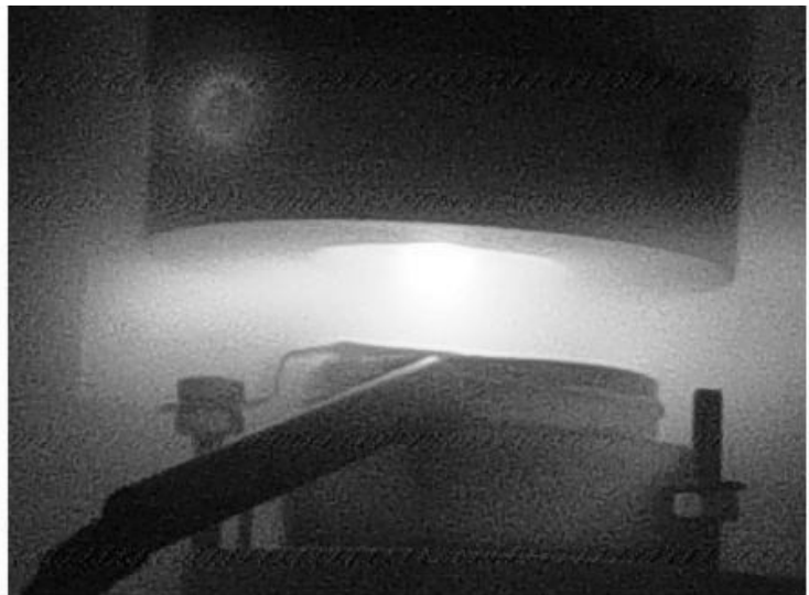
Figure 2. Running discharge in the low-pressure plasma-jet deposition system.
