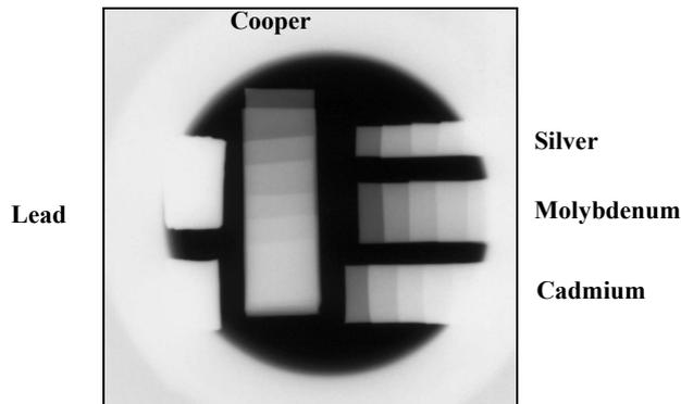
**Fig. 1:** Typical digital computer image of a radiographic film obtained after an effective shot.
