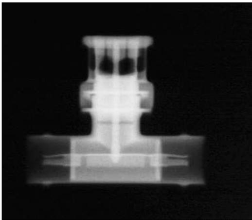
**Fig. 2:** Single X-ray image of a stainless steel BNC T connector .
