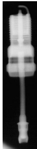
**Fig. 3:** Single X-ray of an spark plug.
