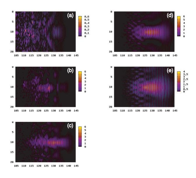
**Figure 1.** The intensities of laser pulses after propagating  $2.5L_{\rm R}$  for electron densities  $n_e=$  (a) 20, (b) 10, (c) 5, (d) 2, and (e)  $1\times 10^{19}{\rm cm}^{-3}$ , respectively.
