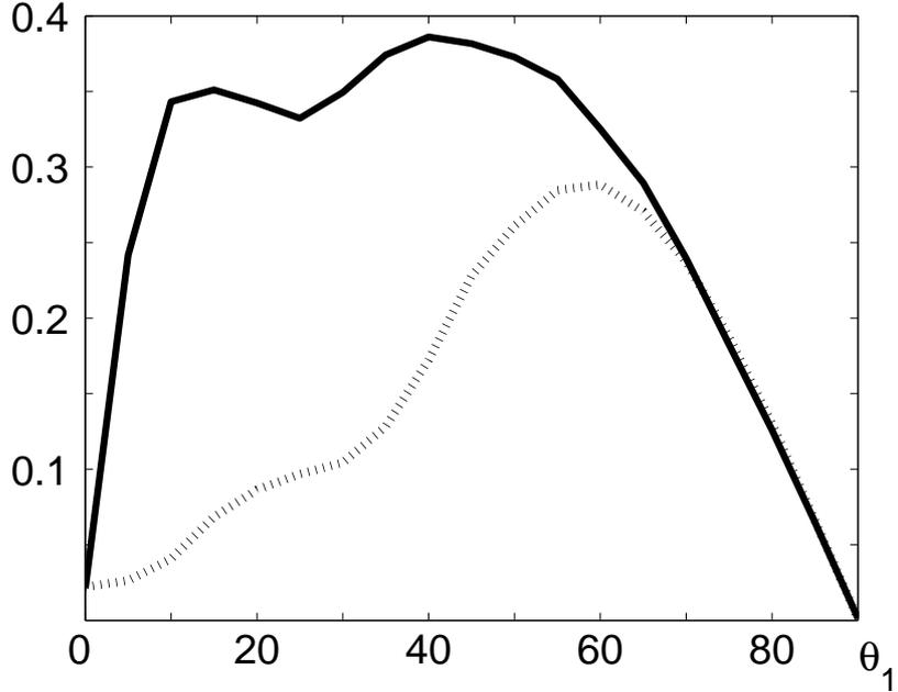
FIG. 3: Averaged electron velocity versus  $\theta_1$  (in degrees) for the one-wave scheme with  $\bar{A}_1 = 0.1$ ,  $\bar{A}_2 = 0$  (dotted lines) and the two-wave-scheme with  $\bar{A}_1 = 0.1$ ,  $\bar{A}_2 = 0.01$  (solid lines) at time  $\Omega t = 7000$ , for low-density runs  $e_0 = 0.3$ .
