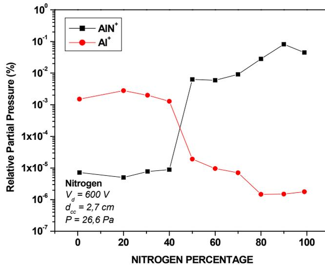
Figure 13. The variation of the aluminum nitrite and atomic aluminum signals as a function of the percentage of nitrogen in the N<sub>2</sub>/Ar gas mixture.
