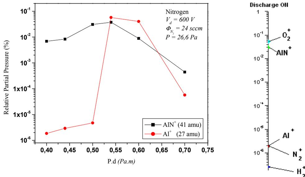
Figure 11. Variation of the Aluminum (27 amu) and AlN<sup>+</sup> (41 amu) peaks for the hollow cathode discharge operating with nitrogen at pressure of 26.6Pa.
