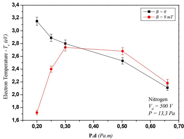
Figure 9. Effect of the magnetic field on the electron temperature at a constant value of the discharge voltage.
