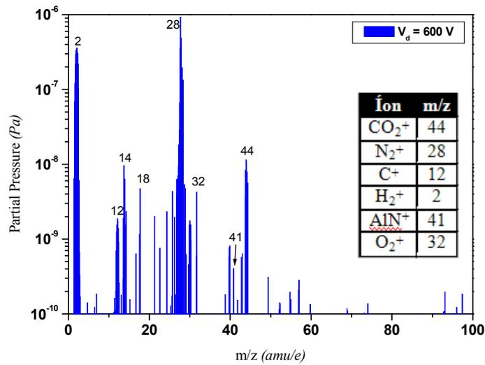
Figure 10. Mass spectrum of the discharge in N<sub>2</sub> for pressure of 13,3 Pa, subtracted from background spectrum.
