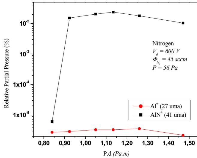
Figure 12. Variation of the Aluminum (27 amu) and AlN<sup>+</sup> (41 amu) peaks with the discharge operating at a nitrogen pressure of 56 Pa.
