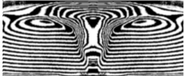
**Fig. 5.** Resultant interferogram transferred back into degrees of shade and modified with a Gaussian filter of size 3x3.
