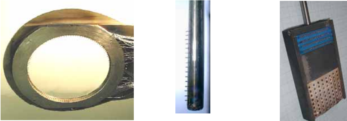
Fig 1. Langmuir probe arrays for spatially resolved measurements. Left - the poloidal limiter equipped with 124 probes; Middle - the rake probe, Right - the 2D matrix of 64 probes.
