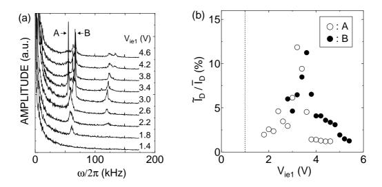
**Figure 3.** (a) Frequency spectra of electron saturation current and (b) normalized fluctuation amplitudes  $\tilde{I}_D/\bar{I}_D$  as a function of  $V_{H1}$  for  $V_{H2}=0$  V and  $V_D=90$  V at r=0 cm in the parallel shear case.
