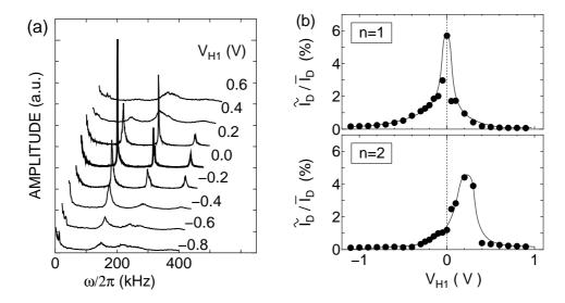
**Figure 2.** (a) Frequency spectra of electron saturation current and (b) normalized fluctuation amplitudes  $\tilde{I}_D/\bar{I}_D$  as a function of  $V_{H1}$  for  $V_{H2}=0$  V and  $V_D=90$  V at r=0 cm in the perpendicular shear case.
