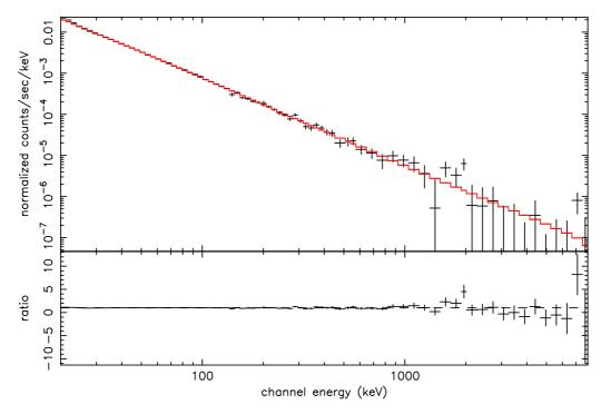
Figure 4. SPI Crab spectrum extracted from 44 NRT science windows in INTEGRAL revolution 44, using OSA 3.0 and a saturated Ge background model fitted detector by detector with Gaussian statistics.
