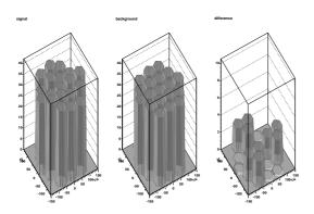
Figure 2. Count rates in the 19 Ge detectors in the 20-8000 keV band, during a Crab on axis pointing. From left to right: total count rate, estimated background count rate and their difference. The pattern of the projection of an on axis source through the mask on the detector plane, with its 120 degrees symmetry, is visible.
