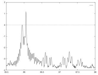
**Fig. 12.** Experimental spectrum, showing the diffracted intensity I(q) in arbitrary units as a function of wave vector q, for a Prouhet-Thue-Morse GaAs-AlAs multilayer with N=128 (courtesy F. Laruelle, L. Leprince and J. Schneck, CNET-Bagneux).
