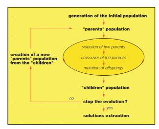
Fig. 1. General scheme of a Genetic Algorithm.
