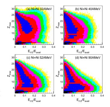
Figure 2: (Color online) Experimental correlations between the size of the largest detected fragment  $Z_{max}$  and the total transverse energy of light charged particles divided by available c.m. energy, for Ni+Ni collisions. A minimum of 4 wellidentified charged particles was required in the off-line analysis. Logarithmic contour levels are shown corresponding to the number of events (darker tones indicate larger numbers).
