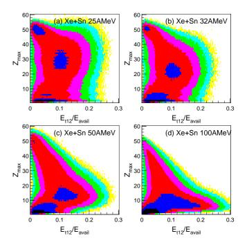
Figure 1: (Color online) Experimental correlations between the size of the largest detected fragment  $Z_{max}$  and the total transverse energy of light charged particles divided by the available c.m. energy, for Xe+Sn collisions. A minimum of 4 well-identified charged particles was required in the off-line analysis. Logarithmic contour levels are shown corresponding to the number of events (darker tones indicate larger numbers).
