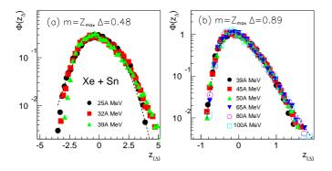
Figure 9: (Color online) (a)  $Z_{max}$  distributions for Xe+Sn collisions at 25–39A MeV, scaled according to Equation 1 with  $\Delta$  given by a linear fit to the data of Figure 8a of the form  $\sigma \sim < m > \Delta$ . The dashed curve is a best fit to scaled data using a Gaussian distribution. (b) As (a) but for bombarding energies 39–100A MeV. The dashed curve is a best fit to scaled data using the Gumbel distribution, Eq.5.
