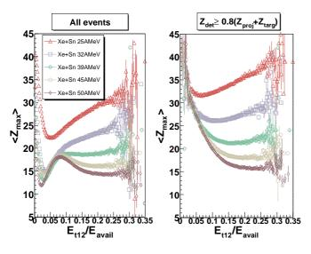
Figure 3: (Color online) The mean charge of the largest fragment detected in each event,  $Z_{max}$ , as a function of the total transverse energy of light charged particles (normalised to the available centre of mass energy) for Xe+Sn collisions between 25 and 50A MeV. Vertical bars show the estimated statistical error on the mean. It should be noted that events with  $E_{t12}/E_{avail} \gtrsim 0.2$  correspond to only 1% of the total measured cross-section.
