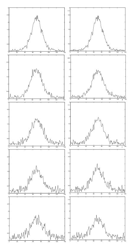
Figure 5: Evolution of the sections at times t=2, 4, 6, 8, 10 for NLS with multiplicative noise with Dirichlet (left) and periodic (right) boundary conditions ( $\sigma = \frac{1}{2}$ ,  $\epsilon = 0.03$ ).
