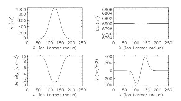
Figure 6: FIG. 6. An example of a deep plasma cavity containing hot electrons (1 keV) surrounded by a cold (1 eV) highly magnetized plasma. See section III.D for details. 25
