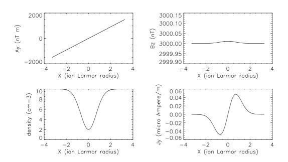
Figure 1: FIG. 1. A deep and narrow density depletion in a highly magnetized plasma. The parameters of this equilibrium are given in Sec. III.A.
