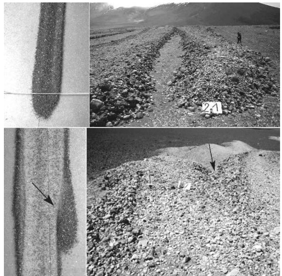
FIG. 15: (top, left) Accumulation of large black particles in the front of laboratory granular flows, and (top, right) accumulation of large pumices in the front of the right lobe, in the Lascar pyroclastic flows deposits. Lobes fingering (bottom, left) in a glass beads flow deposit and (bottom, right) in a Lascar pyroclastic flow deposit (main flow going to the far right). The black arrow shows the point where the flow separates in two lobes. In the left picture, the small flow is particularly rounded in shape and still covered by large particles, because it did not propagate far enough to empty the back of the deposit. There is an accumulation of large black particles and of large pumices in the levées (see also fig. 1, top).
