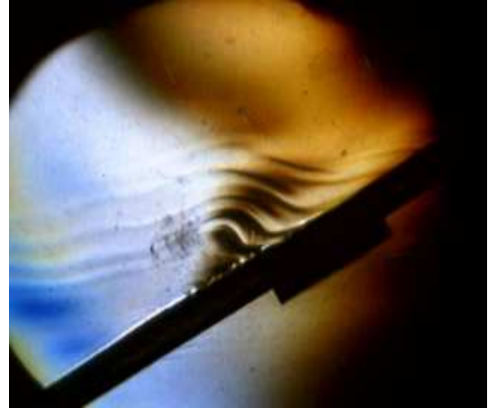
FIG. 5: Isodensity lines during the slightly supercritical reflection ( f/f_c = 1.14 ) of an internal wave on a slope. The slope (thick black line) has an angle \gamma = 35^\circ . The incident wave plane comes in from the left (inclined white region near the top left corner between blue and yellow regions). The reflected wave plane is hardly noticeable. Vibrational parameters: f = 0.32 Hz and A_{pp} = 6.7 mm. This picture should be compared with Fig. 2c. (Color picture).
