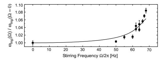
Fig. 2 – Transverse monopole frequency  $\omega_{\rm mp}(\Omega)$  normalized by  $\omega_{\rm mp}(\Omega=0)$  as a function of the stirring frequency  $\Omega$ . For a non rotating condensate  $(\Omega=0)$  we measure  $\omega_{\rm mp}(0)/(2\pi)=130.6$  Hz. The vertical bars indicate the error given by the fitting routine.
