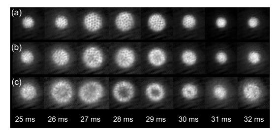
Fig. 1 – Series of images of the condensate for various waiting times  $\tau$  after excitation. Row a) corresponds to a rotation frequency  $\Omega/(2\pi)=62$  Hz, row b) to  $\Omega/(2\pi)=64$  Hz and row c) to  $\Omega/(2\pi)=66$  Hz.
