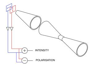
Figure 1. The two detectors in a single PSB share the same optics, but have different readouts.
