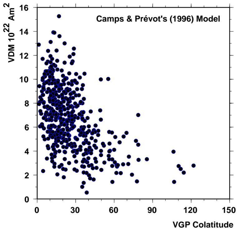
**Figure 12.** a/ VDM for the Brunhes period from the PINT database (open circles) represented as the function of the VGP colatitude and compared to Amsterdam VDMs (Black circles). b/ 500 random simulated VDMs from Camps and Prévot's (1996) statistical model.
