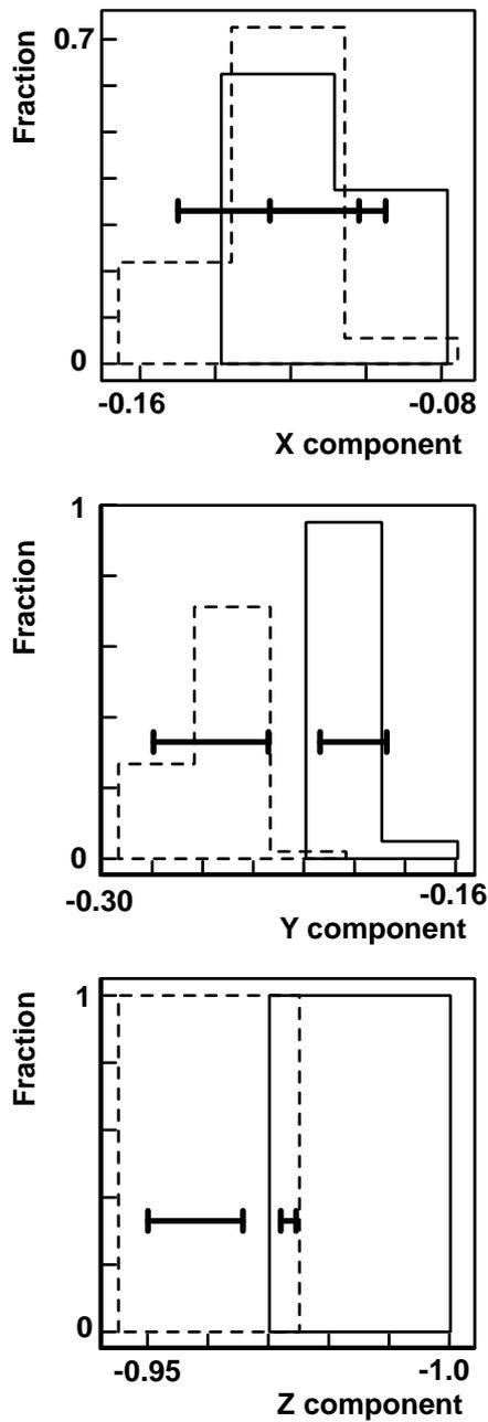
**Figure 3.** The bootstrap test for a common mean direction for flows am1 and am2 (Tauxe, 1998) illustrated by the histograms of the cartesian coordinates of the bootstrapped means for flows am1 (solid line) and am2 (dashed line). Because the 95% confidence intervals for Y and Z components do not overlap, we assume that the two lava flows have a significantly different mean direction.
