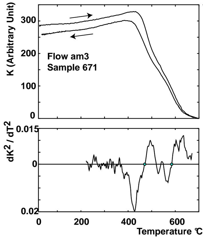
**Figure 4.** Example of thermal variation of weak field magnetic susceptibility  $K$  (measured in induction  $B$  equal to  $100\mu\text{T}$ ) against temperature  $T(^{\circ}\text{C})$  showing a good reversibility and second derivative of the smoothed data of the heating curve. The mean Curie temperature is defined when the second derivative increases to zero (Prévot et al., 1983)
