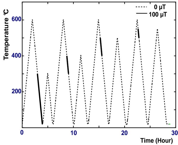
**Figure 6.** Temperature as a function of time for a sample heated and cooled at a constant rate of  $5^{\circ}/\text{mn}$ . The curve shows the succession of pTRM acquisitions in an applied field of  $100 \mu\text{T}$  (solid line) during cooling and demagnetizations (dashed line) carried out during the pTRM-tail test. Parameter A is calculated as the ratio of the intensity of the tail of pTRM normalized by the original pTRM, both measured at room temperature
