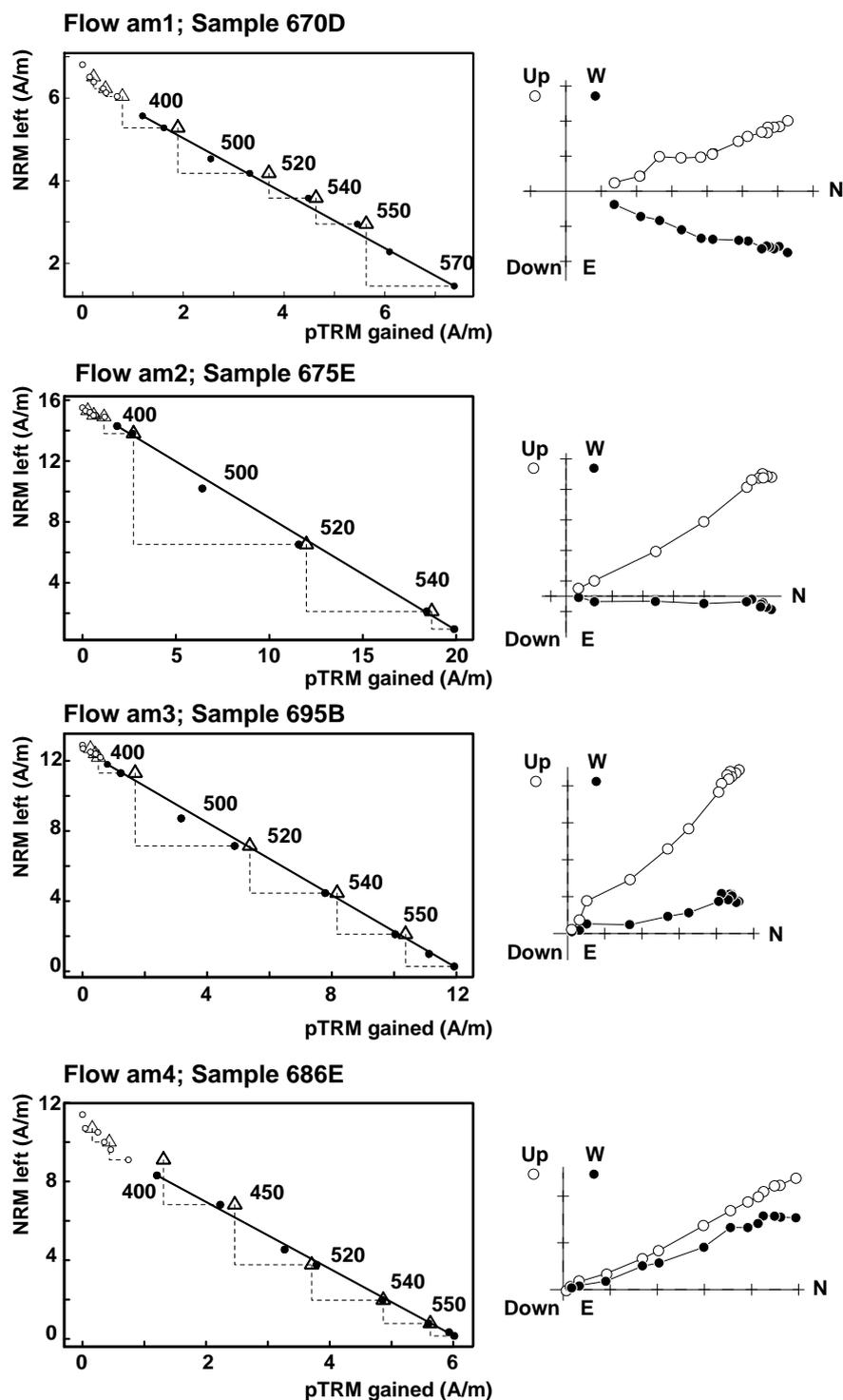
**Figure 8.** Examples of typical Arai plots with the corresponding orthogonal vector projections. On the Arai plots the triangles represent the pTRM checks and solid (open) symbols correspond to accepted (rejected) points. In the orthogonal vector diagrams, solid (open) circles represent projection into the horizontal (vertical) plane.
