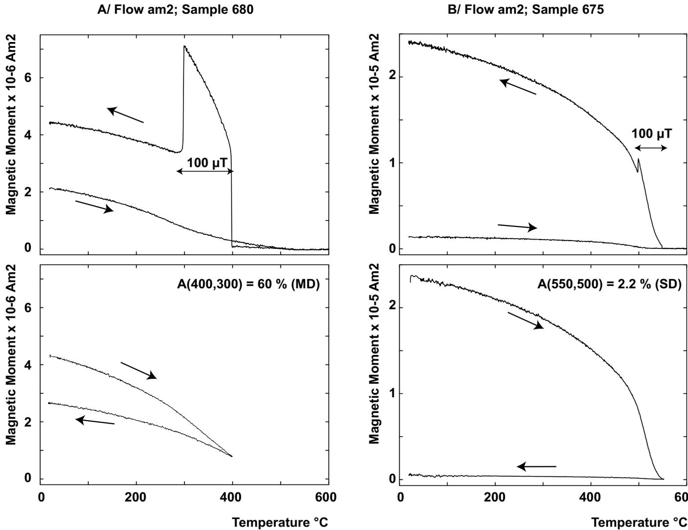
**Figure 7.** Thermomagnetic curves acquired during pTRM acquisition (top) and pTRM demagnetization (bottom). In example A the pTRM is imparted on the interval (400°C-300°C). Subsequent demagnetization to 400°C leaves an important tail. In example B, the pTRM is imparted on the interval (550°-500°C) and is almost completely demagnetized after heating back to 550°C.
