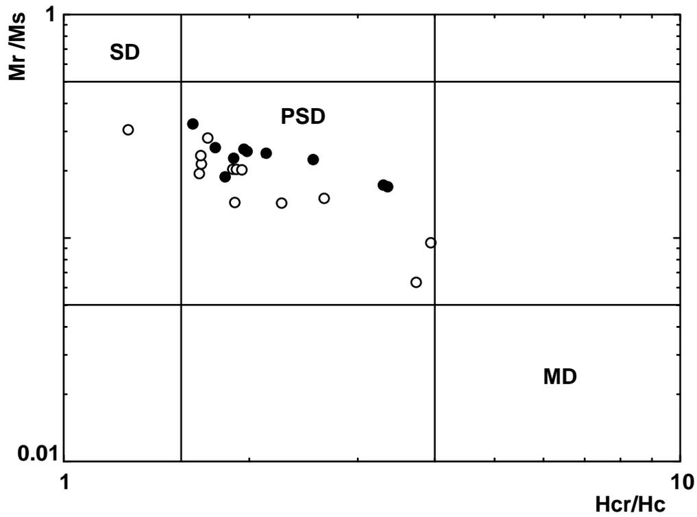
**Figure 5.** Hysteresis parameters ratio measured at room temperature plotted on a log-log scale. Solid (open) symbols correspond to accepted (rejected) samples for paleointensity experiments on the basis of selection and reliability criteria discussed in the text.
