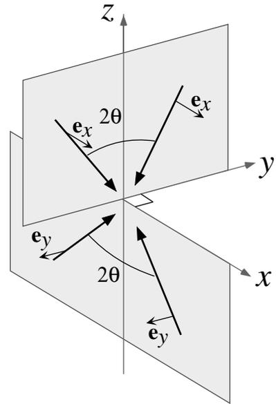
FIG. 1: Beam configuration of the 3D lin  $\perp$  lin optical lattice. Two beam pairs propagate in the  $xz$ - and  $yz$ -planes, and are orthogonally polarized along the  $y$ - and  $x$ -axes respectively. They form an angle of  $\theta = 45^\circ$  with the  $z$ -axis.
