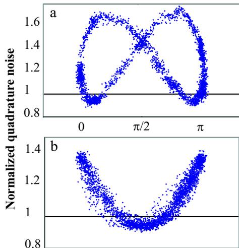
FIG. 5: Normalized quadrature noise for the  $A_y$  mode vs the relative phase between the mean field mode and LO. In curve (b), taken at a noise frequency of  $3MHz$ , quadrature squeezing is achieved when  $\theta_{hd} = \pi/2$ :  $\hat{S}_3$  is squeezed. The general case is shown in curve (a): a linear combination of  $\hat{S}_2$  and  $\hat{S}_3$  is squeezed.
