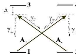
FIG. 1: Schematic energy level diagram for the X-like four-level system:  $\gamma_{\perp} + \gamma_{\parallel} = \gamma$  is the optical dipole decay rate;  $A_{\pm}$  denote the left- and right-circularly polarized components of the light field;  $\Delta$  is the detuning from resonance.
