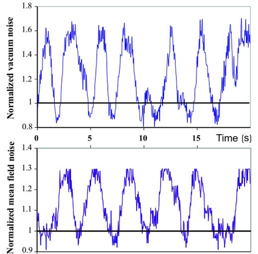
FIG. 4: Normalized quadrature noise for the vacuum field mode ( $A_y$ ) at 3 MHz and for the mean field ( $A_x$ ) mode at 5 MHz. The best squeezing is 5% for the mean field mode and 13% for the vacuum mode.
