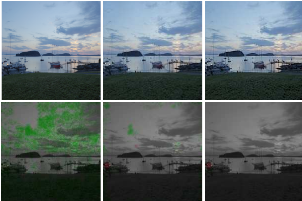
FIG. 3.4. Comparison between the final output with 50 \times 50 and 200 \times 200 neighborhoods. Top left: input tone mapped image of Reinhard et al. [23]. Top middle: final output with 50 \times 50 neighborhood. Top right: final output with 200 \times 200 neighborhood. Bottom row: corresponding distortion maps.
