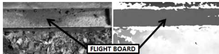
Fig. 1. Couple of intensity (left) / disparity (right) images provided by the stereo vision camera. The beehive is visible on the top. Bees take off/land on the flight board.
