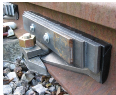
Figure 2: Schrey and Veit rail damper
