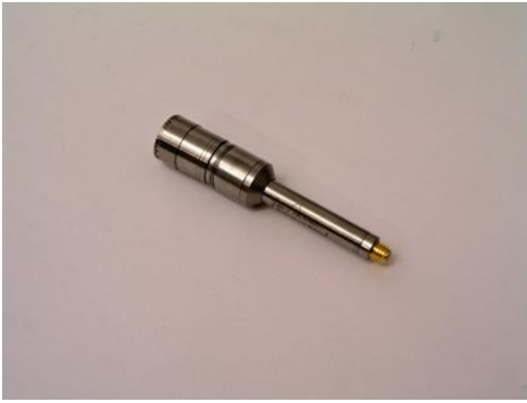
Figure 8: Infrasonic microphone used.
