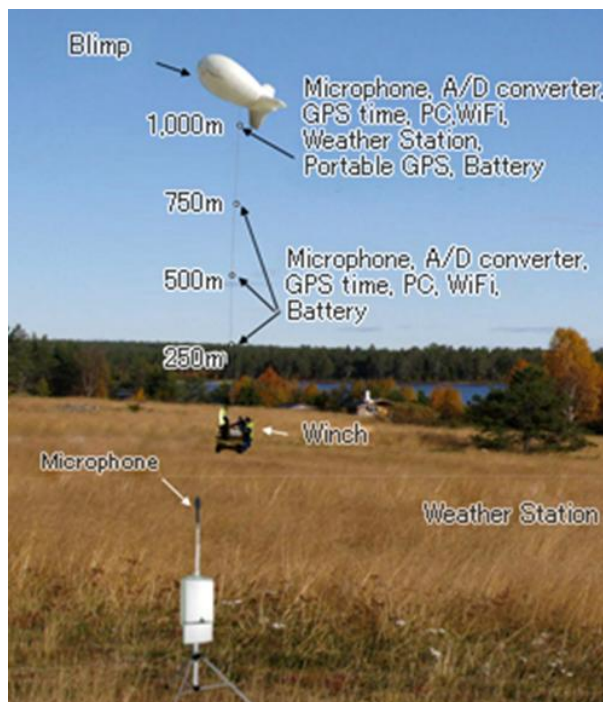
Figure 7: Outdoor measurement systems.
