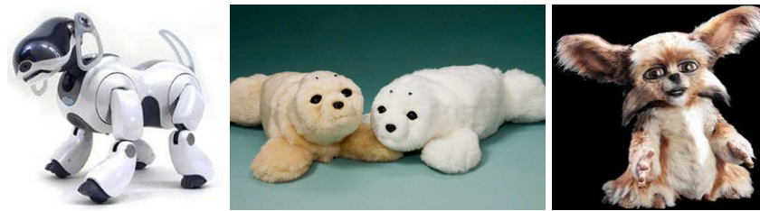
Fig. 2 Examples of zoomorphic social robots, from left to right: Aibo [9], Paro [10] and Leonardo [11].
