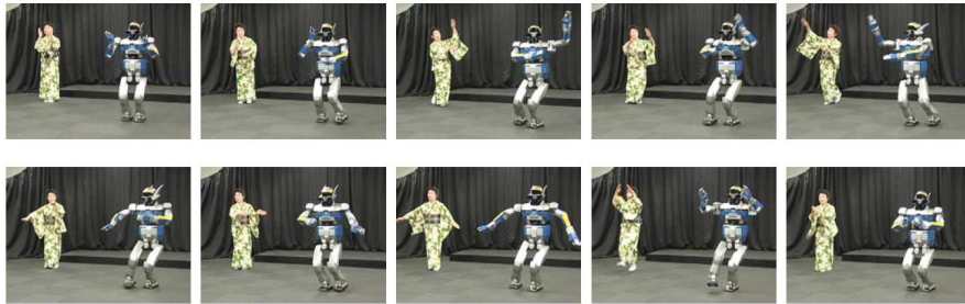
Fig. 13 Humanoid robot performing a Japanese dance. The motion has been generated by retargeting and dynamically filtering human motion capture data (from [56]).
