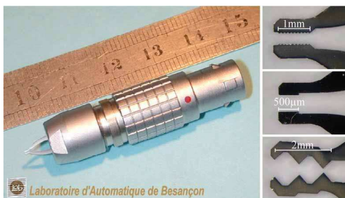
Fig. 2. MMOC Microgripper (left) and finger tips (right).
