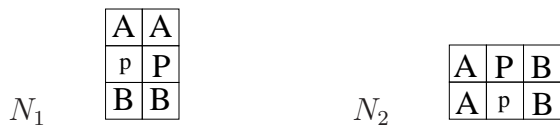
Fig. 14. Non-symmetric masks. No \pi/2 rotations are considered. The labels p and P indicate pixels that must belong to the set P which is a set composed of simple pixels; the label p (lower case) indicates the position of the pixel which is currently examined. At least one of the pixels marked A and at least one of the pixels marked B must be in S .
