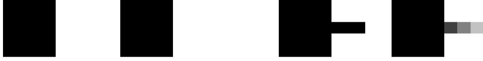
Figure 6: Signal approximation with the two-dimensional total variation: For two piecewise constant images with two values, the estimation may (left case) or may not (right case) recover the correct level sets, even with infinitesimal noise. For the two cases, left: original pattern, right: best possible recovered level sets.
