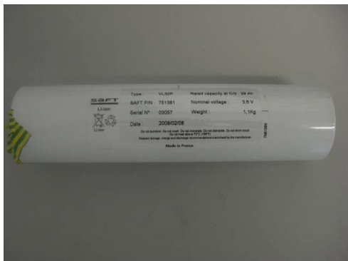
Figure 1: Lithium-ion VL30P cell from SAFT
