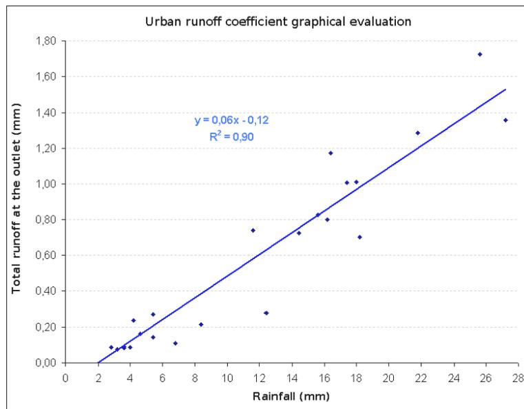
**Figure 5. The angular coefficient of the linear adjusted graphic (total runoff versus precipitation) is an estimation of the urban runoff coefficient. There are 2mm of initial losses over the urban zone according to this graphic.**
