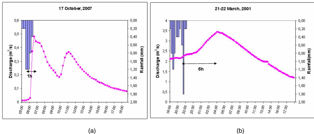
Figure 2. Observed discharge (m<sup>3</sup>/s) in pink lines and averaged 15 min observed rainfall (mm) represented by blue bars on (a) 17 October 2007 and (b) on the 21st -22nd of March 2001. The time-lag is indicated by double arrows.
