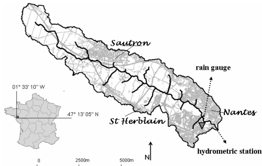
**Figure 1. Chezine catchment indicating the location of the rain gauge and the hydrometric station at the outlet. The grey areas correspond to the urban database layers superposed (roads and buildings).**
