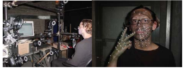
Figure 4: Motion capture using a VICON® system with 12 cameras, 50 beads glued on the hand and 63 on the face.
