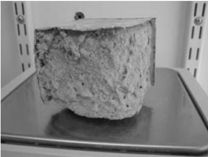
Figure 9b. Picture of a 7 \times 7 \times 7 \text{ cm}^3 sample of FL with 3 faces isolated after cycle 12.
