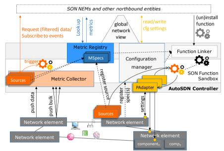
Fig. 3. Functional overview of the AutoSDN controller
