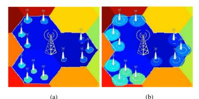
Fig. 6. (*left*) coverage map produced by the simulator with no SON functions; (*right*) increased CRE of the picos after activation of the LB SON
