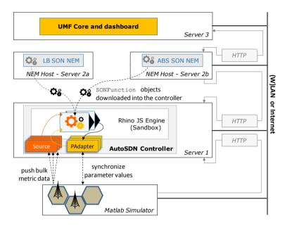
Fig. 4. System view of the AutoSDN prototype setup
