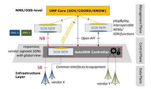
Fig. 1. High level AutoSDN architecture
