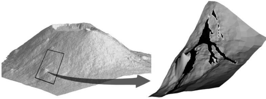
Figure 7: Digital elevation model of the Piton de la Fournaise volcano in 2008, with a 5 meter horizontal resolution (left). Zoom with the observed arrested flow contours (right).
