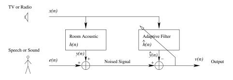
Figure 2: Block diagram of an echo cancellation system
