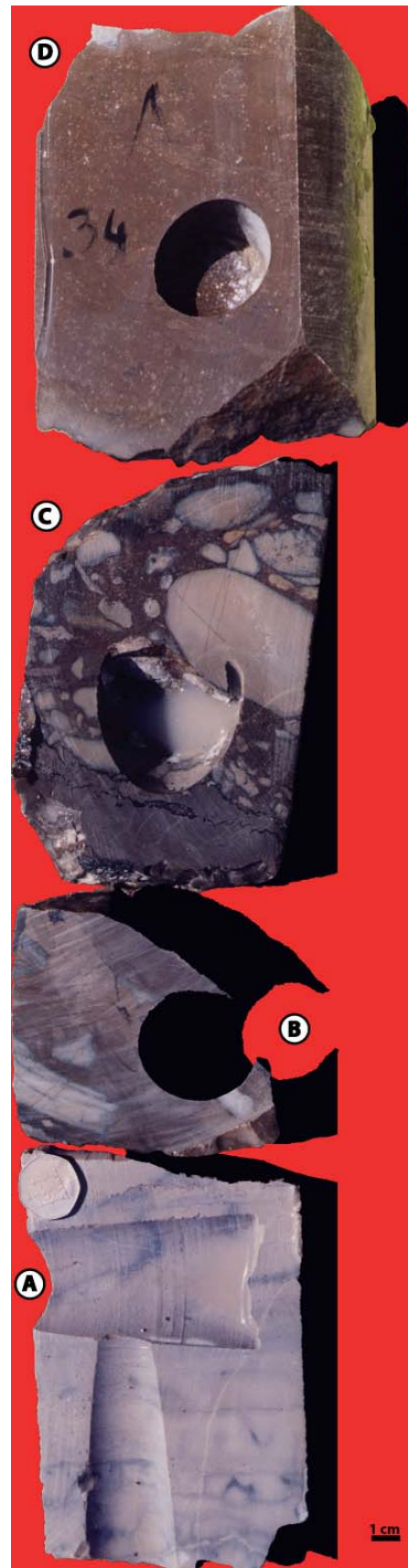
Figure 17: A set of 4 core slabs illustrating the Habshan - Bu Haseer boundary, well N° IFI of field 'X', offshore Abu Dhabi. Slab A: vermicular mudstone of the Habshan; slabs B and C: lag deposit, which forms the extreme base of the Bu Haseer unit, with characteristic pebbles and cobbles; slab D: fossiliferous wackestone.
