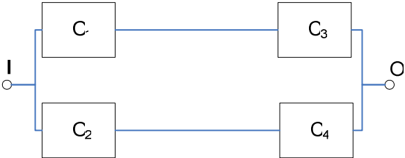
Fig. 3 : Equivalent reliability diagram if C5 = Down
