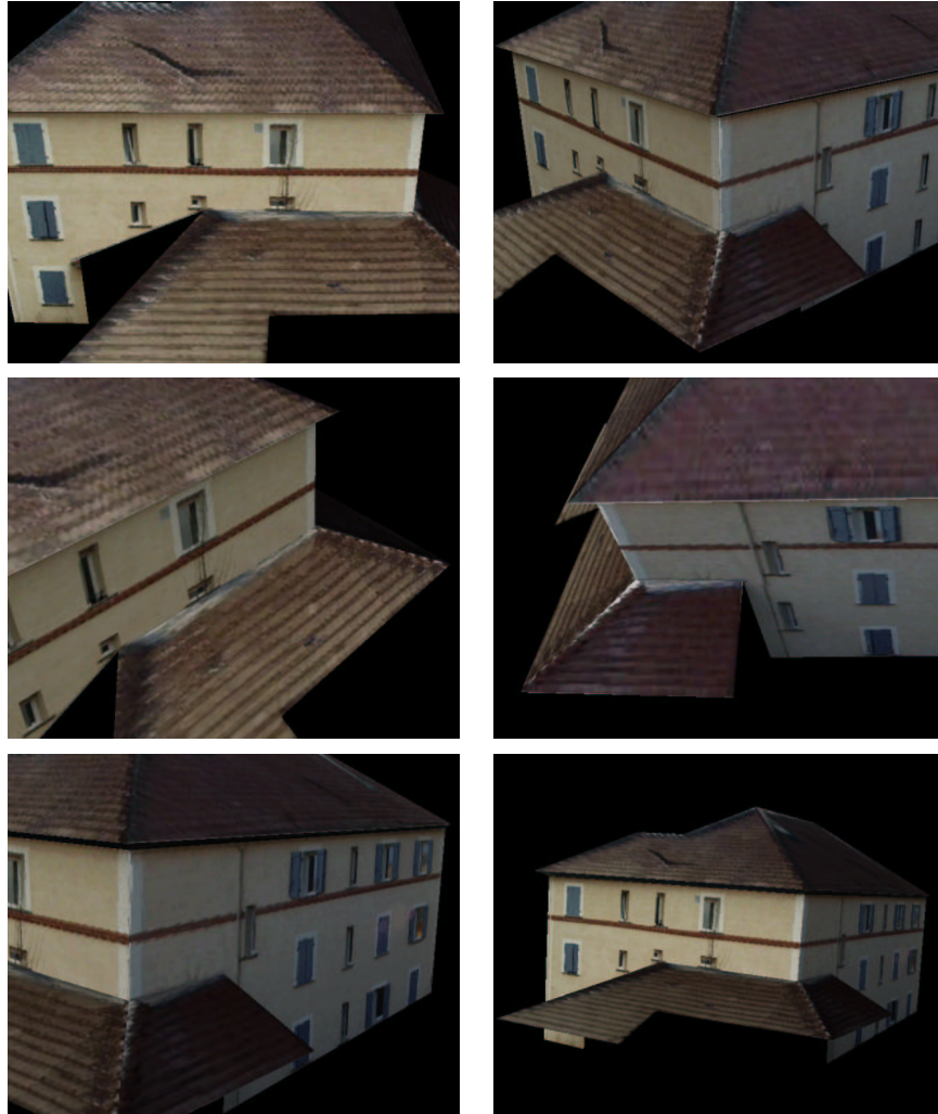
Figure 6: Different views of the textured model. Note that artefacts may be induced by possibly unmodeled non-planar parts of the surfaces, e.g. the pole bulging out of the roof in the top-right image is wrongly mapped to the roof plane, and is therefore distorted in other views, e.g. the top-left one.
