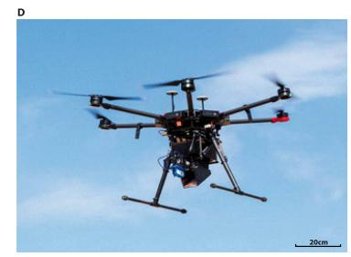
Fig. 1. The adult mosquito release system operated from an UAV. (A) Front right view of the release mechanism (technical drawing). (B) Half-section of the release mechanism (technical drawing). (C) Canister filled with 50,000 marked mosquitoes. (D) Fully assembled aerial mosquito release system attached to a DJI M600 UAV in flight.
