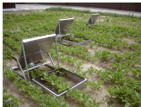
Measurement of  $N_2O$  and  $CO_2$  fluxes with automatic chambers in a sugar beet plot, Estrees-Mons, June 2008 bessou©INRA
