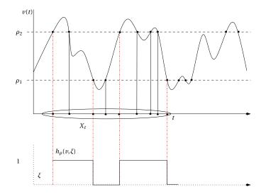
Fig. 2.7. **Definition of the relay filtering for continuous signals**. The set  $X_t$  is intended for identifying the times where the relay switches; similarly to the discrete relay, this operation allows to identify the oscillations of v which cross in the interval  $[\rho_1, \rho_2]$ .
