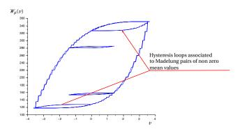
Fig. 2.26. Outputs of the Preisach plotted under the form of a Lissajous diagram. In this case, the distribution of weights  $\mu_i$  is not symmetrical with respect to the straight line  $\rho_1 + \rho_2 = 0$  and the contribution to the total variation of  $\mathcal{W}_{\mu}(v)$  of the hysteresis loops associated to the Madelumg's pairs depends on their mean values.
