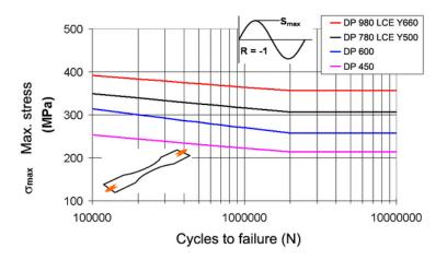
Fig. 1.10. Example of tension-compression Wöhler curves (Arcelor-Mittal). These curves are measured at mean stress  $\sigma_m = 0$ , for three different materials. This figure shows poorness of the tests performed to characterize the material fatigue behavior: We will see in the following that lifetime simulations carried out on a complex structure with this kind testing results don't lead to relevant results.
