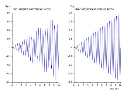
Fig. 3.3. **Integration of an undamped oscillator at resonance.** The figure Fig.a shows the effect of a sub-sampling of the excitation with respect to the characteristic frequency of the convolution kernel. Note on the other hand (on the figure Fig.b) that the numerical integration by convolution allows to accurately reproduce the divergence of the solution of a second order equation excited at the resonance.
