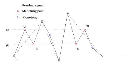
Fig. 1.14. Illustration of the simplification processes applied in the rain-flow algorithm. The blue samples are removed by an argument of monotony while red samples (which are Madelun's pairs) allow to count the oscillations of magnitude  $\frac{\rho_2 - \rho_1}{2}$  at average  $\frac{\rho_2 + \rho_1}{2}$  which are present in the signal. The residual signal, in dashed line, will in turn be post-processed by duplication of the signal, see figure (Fig. 1.15).
