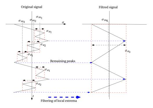
Determination of alternating and mean stresses
