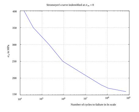
Fig. 1.18. Identification of Stromeyer coefficients obtained from the experimental data given in table Tab 1.1.
