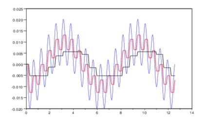
Fig. 2.15. **Representation of**  $t \mapsto \mathscr{E}(v, t, \sigma_a)$  **(bold lines) for some values of**  $\sigma_a$ . The curve in blue is the input signal; the filtering effect increases with  $\sigma_a$ . Further note that regularization of equation (2.39) rounds the outputs, which are theoretically rectangular.
