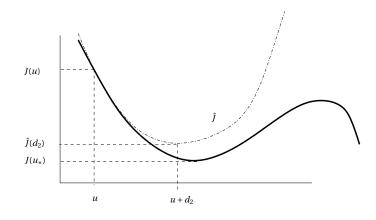
Fig. 4.4. Second order approximation of J. The functional J (in boldline) and its second order approximation  $\hat{J}$ , in dashed line. The Newton step  $d_2$  is the increment which must be added to u to obtain a minimizer for  $\hat{J}$ .
