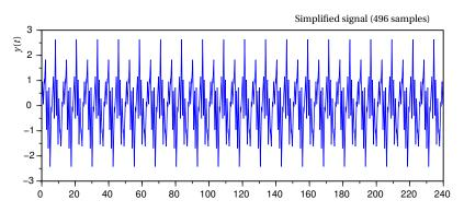
Fig. 1.21. Simplification of the original signal in removing the monotone sequences.
