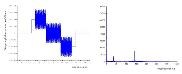
Fig. 4.18. **Torques applied to the ends** *A* **and** *E* **of the beam**. They contain the frequencies 35, 137 and 145 which permit to excite the first eigen-modes of the beam, depicted in figure (Fig. 3.8) page 111.
