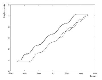
Fig. 2.37. **Hysteresis loop for the Coulomb's damping.** The reader should compare this result with the one that would have been obtained with linear dissipation (ie. if the Rayleigh dissipation is quadratic function of velocity).
