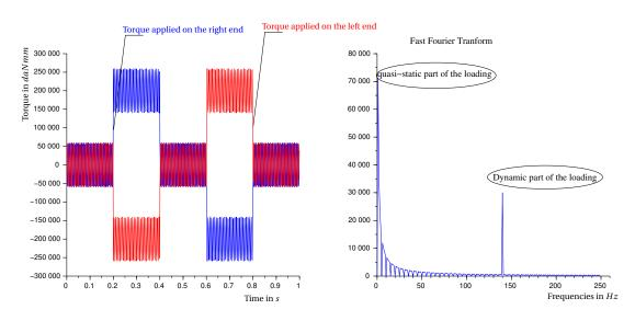
Fig. 3.10. **Dynamic loading of the beam.** As in the case shown on the figure (Fig 3.9.a) the beam is loaded at points *A* and *E* by two opposite torques; the magnitude of the pulsed torque at 140 *Hz* is about 40% of the quasi-static loading.
