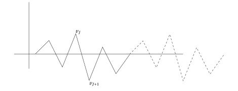
Fig. 1.15. Generic shape of a residual signal obtained at the end of the rain-flow-algorithm. The number of cycles of the residual signal is computed with the help of the rain-flow algorithm by processing the signal obtained by concatenating the points of the solid line to those of the dotted line curve. And this is precisely the purpose of the counting function  $a^{per}$ .
