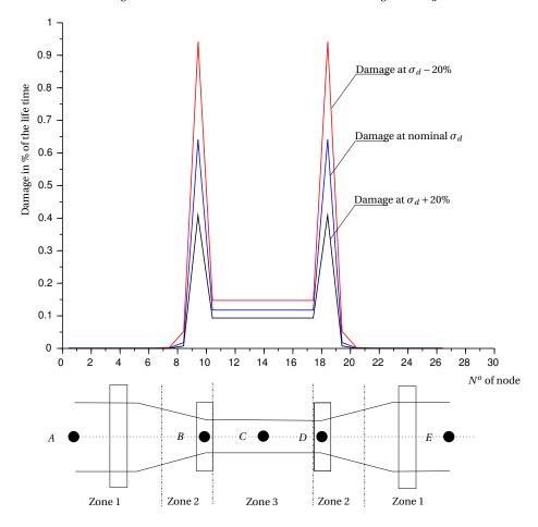
Damage calculated on the beam for different values of the fatigue limit  $\sigma_d$
