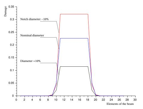
Fig. 3.15. **Quasi-static simulations**. In this case, only the modifications that affect the stiffness of the beam have an effect on the damage, and this justifies to compute the damage with the help of dynamic simulations.
