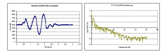
Fig. 1.2. Example of mission profile "3 bumps crossing". The spectrum of the signal (on right) doesn't contain high frequencies and the response of the structure can be assumed to be quasi-static. Loading (on left) can, however, cause permanent plastic deformations at the connecting points between body and axles to justify non-linear quasi-static simulations.
