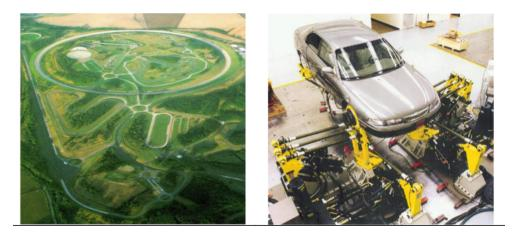
Fig. 1.1. **Example of test bench for fatigue analysis**. The mission profiles are measured on an endurance runway (on the left) and reproduced on a test bench until failure. The most damaging mission profiles are plotted in figures (Fig. 1.2) and (Fig. 1.3)
