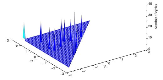
Fig. 1.23. Rain-flow matrix obtained in applying the rain-flow algorithm on the signal shown in figure Fig. 1.21.
