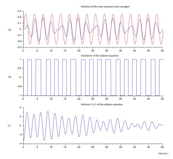
Fig. 4.10. **Details of the resolution of the adjoint equation**. Since in this case their is no bases change to do, the computations are made with a simplified version of the algorithm 4.8. Notice on the other hand that the excitation of the adjoint equation jumps a discontinuity every time the sign of  $\xi_1(t) - \sin \alpha_1 t$  changes and the solution of adjoint system never reaches a stationary state. This justifies the interest of the forced response method introduced in the chapter 3.
