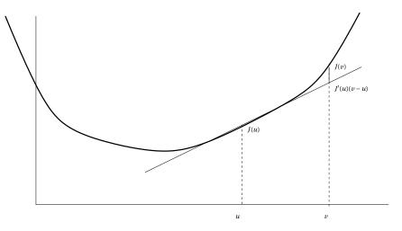
Fig. 4.21. **Geometric interpretation of the inequality** (4.82). The function is located above it's tangent plane.
