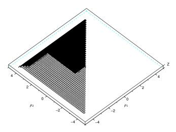
Fig. 2.27. State of the relays at the end of the first loop. The two initializations of the relays plotted in the figure (Fig. 2.25) lead to the same result at the end of the first computation loop, these sates of the relays are used to compute the outputs of the operator  $W_{\mu}$  defined by formula (2.25) page 50.
