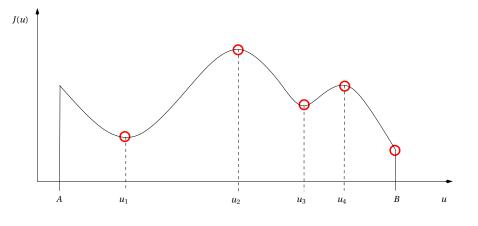
Fig. 4.3. Solutions of the variational inequality (4.5). On this picture, the mapping  $u \mapsto J(u)$  is non convex, defined on the interval [A, B]. The points  $(u_i)_{i=1}^4$  and B are solutions of (4.5), J reaches a local minimum at  $u_1$  and  $u_3$ ; these points can be characterized by the second statement of the Remark 4.3.
