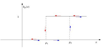
Fig. 2.9. Hysteresis diagram for the relay operator. When v(t) goes increasingly from  $v(t_0) < \rho_1$  to  $v(t_1) > \rho_2$ , the relay  $h_\rho(v)$  switches between 0 and 1, along the blue arrows; next when v comes back decreasingly from  $v(t_1)$  to  $v(t_0)$ , the state of  $h_\rho(v)$  passes from 1 to 0 following the red arrows.
