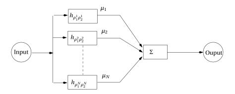
Fig. 2.3. Representation of a Preisach operator for a discrete measure. In this case, the Preisach operator can be understood as an electronic device which is made up of switches connected in parallel with the weights  $\mu_i$ .
