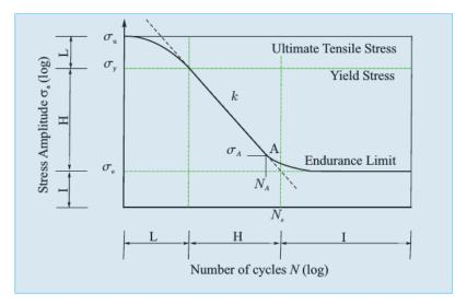
Fig. 1.20. Physical interpretation of the parameter  $\sigma_u$  in Weibull and Stüs-Philips formulas.
