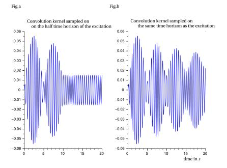
Fig. 3.4. Integration of a damped oscillator (1% of the critical damping) The figure Fig.a shows the effect of a reduction of the time horizon on which the convolution kernel is sampled; the response of the oscillator is over-damped.
