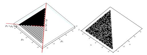
Fig. 2.23. **Initialization of the relays operators.** The relay operators are uniformly distributed in the half Preisach plane; on the left hand diagram they are initialized at 1 if  $\rho_2 + \rho_1 < 0$  and at 0 if  $\rho_2 + \rho_1 > 0$ , while on the right hand one they are randomly initialized.
