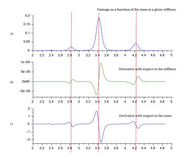
Fig. 4.16. **Damage and its derivatives computed for a given stiffness.** In this case, we fix the stiffness at a given value  $k_0$  and we plot on the figures *a*), *b*) and *c*) the mappings  $m \mapsto \mathcal{D}(k_0, m)$ ,  $\partial_k D(k_0, m)$  and  $\partial_m D(k_0, m)$ .
