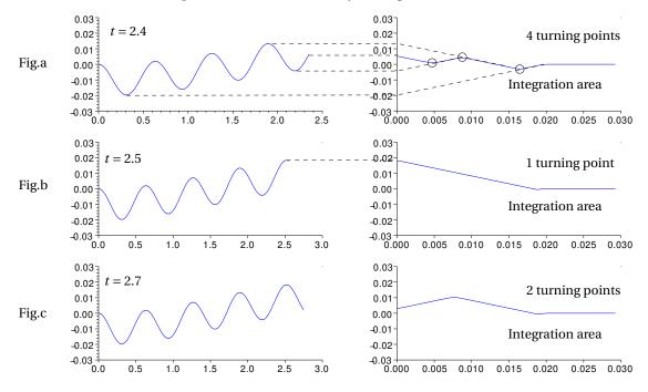
Fig. 2.16. **Representation of**  $\sigma_a \mapsto \mathscr{E}(v, t, \sigma_a)$  **at** *t* **given**. Comparison between the figures Fig.a and Fig.b shows that all or part of the memory of the Preisach operator is erased when the signal reaches an extremum. We will see that this phenomenon causes the non-differentiability of the outputs of the Preisach operator with respect to the inputs.
