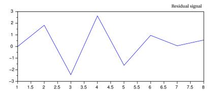
Fig. 1.22. Example of residual signal obtained at the end of the rainflow algorithm.
