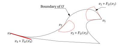
Fig. 4.6. **Cone of feasible directions**. We see on this picture that if v is in the interior of U any direction of E is a feasible direction. When v is on the boundary of U the cones of the feasible directions at the points  $v_1$  and  $v_2$  are surrounded by red lines. For  $v = v_3$  the cone of feasible directions reduces to 0 and we represent on this picture the tangent cone to U such as defined in figure (Fig. 4.7).
