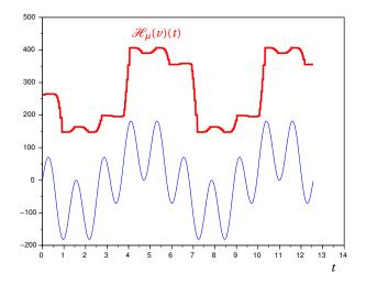
Fig. 2.28. We show on the same picture the output of the Preisach operator and the input 50 \* v (for scaling reasons).
