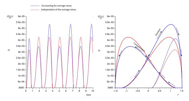
Fig. 2.21. Computation of  $t \mapsto w(v(t), \sigma_0(t), \dot{v}(t))$  in case of the Strohmeyer's formula, with and without mean stress effect, when v(t) is a pure sine. Note that insofar as each cycle is decomposed into sub-elements where the signal v is monotone, we account the parts of the cycle which are in tension (ie.  $\dot{v} \ge 0$ ) in a different way than these which are in compression; this case is plotted on the curves in blue.
