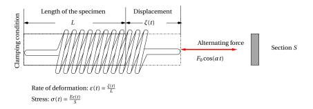
Fig. 4.11. **Mechanical parameters**. Assume that the specimen is submitted to tension-compression loaded by a force  $f(t) = F_0 \cos(\alpha t)$ , we want define the mass-stiffness ratio  $\omega = \sqrt{\frac{k}{m}}$  which minimizes the damage  $\mathcal{D}(\omega)$  when the number of cycles to failure is given by a stromeyer formula (without accounting of mean stress effect).
