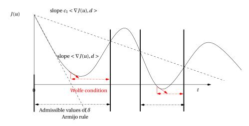
Fig. 4.5. Backtracking method for the line search step. The Armijo condition
