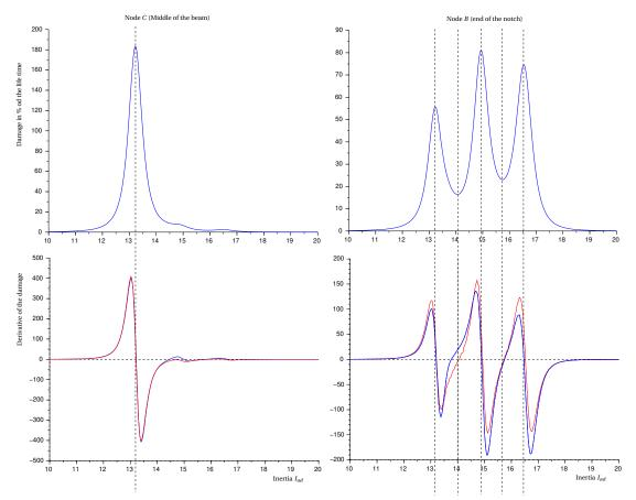
Fig. 4.19. **Comparison between the gradients obtained by integration of the adjoint equation and finite differences**. The curves in red correspond to the computations by finite differences while the curves in blue are the results obtained in solving the adjoint equation.
