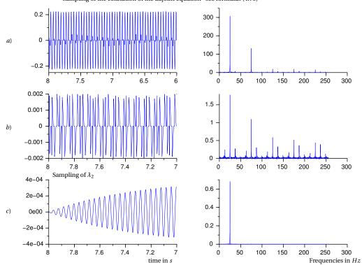
Fig. 4.13. Detail of the computations for the resolution of the adjoint equation in the case of the Example 4.9. We see that the spectrum of the excitation of the adjoint equation is richer than that of the state equation, which contains only one frequency.
