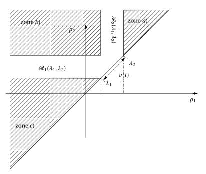
Fig. 2.8. Partition of the Preisach plane in zones where the relay operators are constant. If  $\lambda_1 \leq v(t) \leq \lambda_2$  for  $t \in [t_1, t_2]$  then the mappings  $t \mapsto h_{\rho}(v, \xi)(t)$  are constant if  $\rho$  is in one of the hatched zones, while they vary between 0 and 1 when  $\rho$  lies in one of the strips  $\Re_i(\lambda_1, \lambda_2)$  for i = 1, 2.
