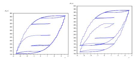
Fig. 2.25. **Outputs of the Preisach plotted under the form of a Lissajous diagram**. The computations are carried out on the signal  $v^{per}$ , which is defined on [0,26*s*], see figure (Fig. 2.22). On the left hand diagram the relay operators are initialized in the standard way while in the left hand diagram the relays randomly initialized. We see that after an initialization phase, the outputs of the Preisach operator are a periodic; this is explained in figure (Fig. 2.27).
