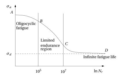
Fig. 1.7. **Generic form of a Wöhler's curve**. We are mainly interested by the part *BCD* of this curve, in other words, we will assume that the applied loading is low enough to ensure lifetime greater than  $10^5$  cycles. In this case, failure is not accompanied with overall plastic deformation. However, permanent plastic deformation due to the first loading cycles can occur.
