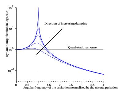
Fig. 3.2. Evolution of  $a(\omega_0)$  as a function of *c*.
