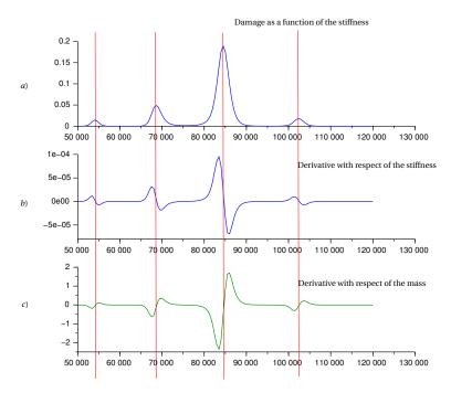
Fig. 4.15. **Damage and its derivatives computed for a given mass**. In this case, we fix the mass at a given value  $m_0$  and we plot on the figures *a*), *b*) and *c*) the mappings  $k \mapsto \mathcal{D}(k, m_0)$ ,  $\partial_k D(k, m_0)$  and  $\partial_m D(k, m_0)$ .
