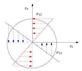
Fig. 3.7. **Stresses in the cross sections of the beam.** When the cross section of the beam is circular, the stresses are maximal in norm on the boundary of the cross sections; but this is generally false for other shapes of the cross section (think for instance to a L shaped cross section).
