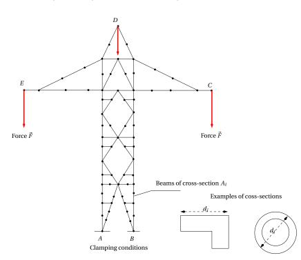
Fig. 4.8. **Example of beam structure**. In this case the electric post is made up of 90 beam elements, it is loaded by given forces  $\vec{F}$  at points *C*, *D*, *E*, which are accounting for the weight of electrical cables.
