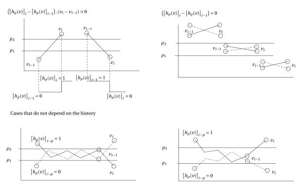
Fig. 2.4. **Proof of the monotony of relay operators.** We must check that  $([h_{\rho}(v)]_i - [h_{\rho}(v)]_{i-1}) \cdot (v_i - v_{i-1}) \ge 0$ ; the 12 scenarios plotted in the figure above should be considered. We plots in the column on left the scenarios that lead to  $([h_{\rho}(v)]_i - [h_{\rho}(v)]_{i-1}) \cdot (v_i - v_{i-1}) > 0$  and in the column on right those which lead to  $[h_{\rho}(v)]_i - [h_{\rho}(v)]_{i-1} = 0$ .
