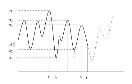
Fig. 2.10. **Definition of a** *RMS* **sequence**. It is a sequence made up of local extrema  $\eta_1, \alpha_1, \dots, \eta_n, \alpha_n \dots$ , listed so that the sequence  $(\eta_i)_i$  is a decreasing sequence of maxima and  $(\alpha_i)_i$  is an increasing sequence of minima.
