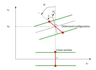
Fig. 4.22. **Mechanical meaning of the Timoschenko's parameters**. In their deformed configuration, the cross-sections of the beam remain plane but they are not necessarily orthogonal to the deformed configuration of the neutral line so that the angle  $\gamma$  measure a shear strain due to the normal loading.
