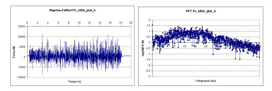
Fig. 1.3. Example of mission profile "Cobbled runway". While remaining at a fairly low level, the excitation spectrum (on the right) can be energetic at high frequencies (frequency range 10 - 40Hz) which may justify of linear dynamic simulations to reproduce the over-stresses resulting from excitability of the body natural modes such as global torsion or bending modes.
