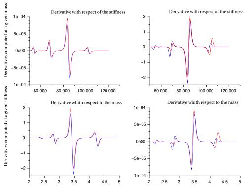
Fig. 4.17. **Comparison between the gradients obtained by integration of the adjoint equation and finite differences**. The curves in red correspond to the computations by finite differences and the curves in blue are the results obtained by resolution of the adjoint equation.
