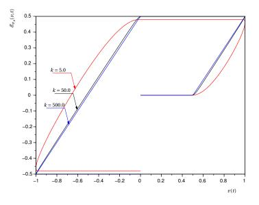
Fig. 2.32. Hysteresis loops for several values of the slope k. In this case the integration is carried out for k = 5.0 (red), k = 50.0 (black) and k = 500 (blue). The integration step is chosen small enough to suppose the outputs of Euler's method converged to the exact solution of the equation (2.48).
