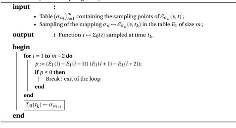
Algorithm 3.3: Computation of the damage caused by a sampled signal  $(v(t_i))_{i=1}^n$ , defined on a time interval [0, T].
