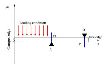
Fig. 4.23. **Beam bending under unilateral constraints.** We are considering a beam of neutral axis  $x_1$ , clamped at the end  $x_1 = 0$  and free at  $x_1 = L$ . We assume that two mountings are installed around the beam to impose the displacements  $x_2(l_1) \ge 0$  and  $x_2(l_2) \le 0$ . The beam is at last loaded by a distributed system of forces  $f(x_1)$  directed along the axis  $x_2$  and non zero for  $0 \le x_1 \le l_1$ .
