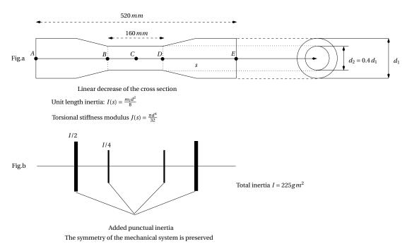
Fig. 3.6. **Description of the mechanical device**. It is a beam of variable cross-section, whose geometric parameters are shown on the figure Fig.a). It is discretized into 26 elements, and submitted at its ends to two opposite torques about the neutral line. We add moreover the 4 punctual inertia shown on the figure Fig.b).
