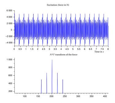
Fig. 4.14. Excitation force in case of the Example 4.10. In this case is the force is  $F(t) = f_0 \cos(\omega_0 t) + \frac{2}{3} f_0 (\sin(1.1\omega_0 t) + \sin(0.9\omega_0 t)) + \frac{1}{2} f_0 (\sin(1.2\omega_0 t) + \sin(0.8\omega_0 t))$ , where  $\omega_0$  and  $f_0$  are given constants; they are sampled on 8 seconds.
