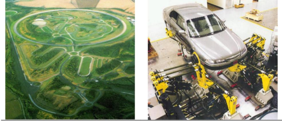
Fig. 1.1. **Example of test bench for fatigue analysis.** The mission profiles are measured on an endurance runway (on the left) and reproduced on a test bench until failure. The most damaging mission profiles are plotted in figures (Fig. 1.2) and (Fig. 1.3)
